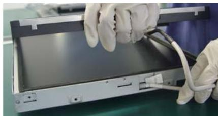
Fix touchbezel to monitor frames with screws.
