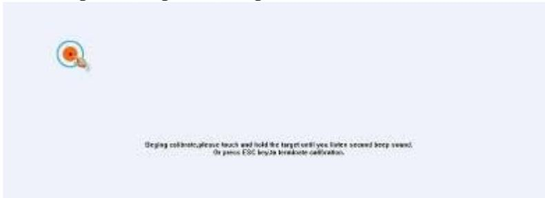
Press the center of red point for about 2-3 seconds. Don't release your finger until the red point shaft to next position or hearing beep sound. Repeat for all red point to finish calibration.
