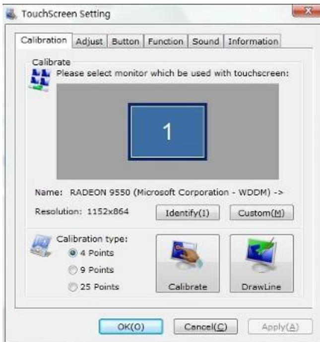
Calibrate: show monitor and resolution information recognized by system
