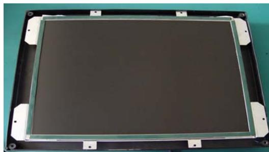
Tear off the outer strips for about 3 or 4mm
